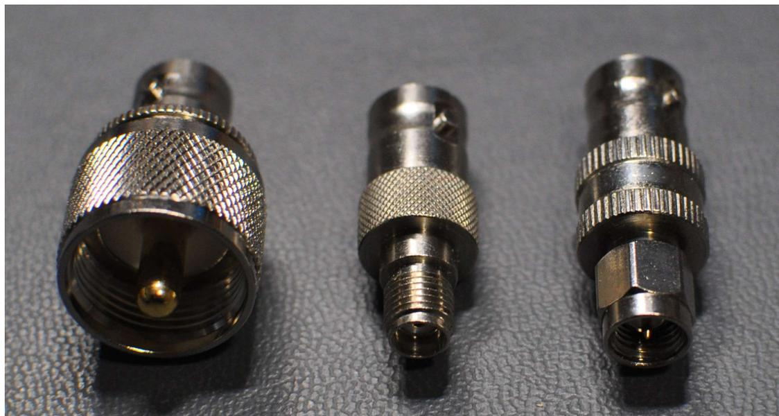
Figure 6: Adaptateurs BNC (UHF, RP-SMA, SMA)
